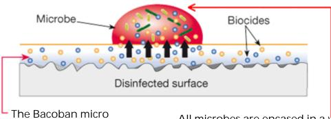
The Bacoban micro thick layer containing the biocides
